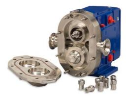
Alfa Laval rotor wings (pistons) rotate around the circumference of the channel in the pump casing. This continuously generates a partial vacuum at the suction port as the rotors unmesh, causing fluid to enter the pump. The fluid is transported around the channel by the rotor wings, and is displaced as the rotor wings re-mesh, generating pressure at the discharge port. Direction of flow is reversible.
