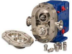
Alfa Laval rotor wings (pistons) rotate around the circumference of the channel in the pump casing. This continuously generates a partial vacuum at the suction port as the rotors unmesh, causing fluid to enter the pump. The fluid is transported around the channel by the rotor wings, and is displaced as the rotor wings converge, generating pressure at the discharge port. Direction of flow is reversible.
