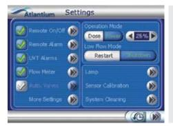
Settings parameters: if set value is exceeded, system delivers error message and alarm.
