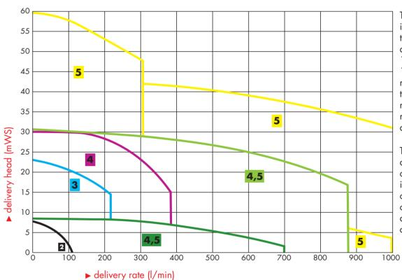
The RM-TS series includes pumps from the RM2-TS type with a delivery rate of 110l per minute, 10 mwc and a 90 W motor to the RM5-TS type with a delivery rate of 1,500l per minute, 60m wc and a 15 kW motor.
